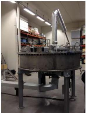
The MicroFuel reactor. This consists of a turntable in which woodchips are exposed to microwaves. This causes flash pyrolysis, leaving bio-char, with the resulting gases condensed to harvest bio-oil.
