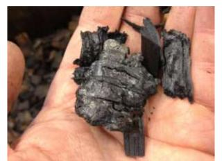
Bio-char produced in the prototype plant. The waste wood has been fully pyrolysed, leaving light carbonized chips © The MicroFuel Project Consortium
