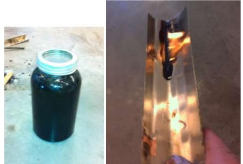
Bio-oil collected from the pyrolysis process (left). It can ignite, confirming its potential as a fuel (right).
